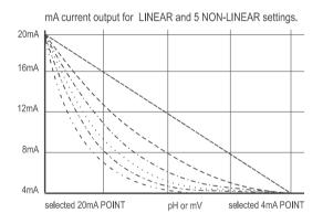
FIG 19 Non-linear effects with 4-20mA current output
