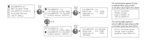
FIG 7 Calibration menu for mV. (ORP)
