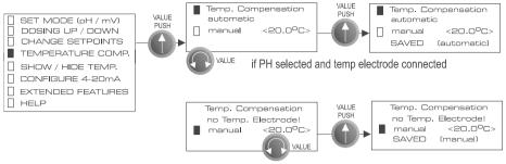
Automatic compensation is only available if a TP-150 temperature electrode is connected.
