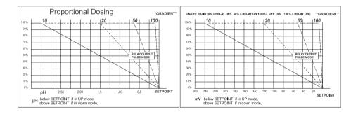
FIG 18 The effect of gradient on proportional dosing
