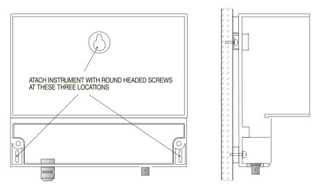
FIG 3 Attaching the DPH-64 to a wall
