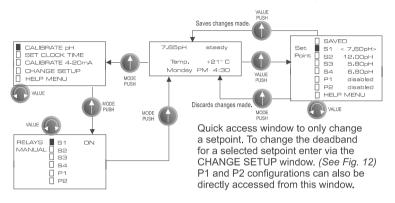
FIG 4 Functions accessible from the main window.
