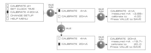
FIG 9 Calibrating 4-20mA current output.
