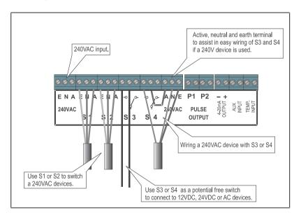
FIG 23 Wiring options for the DPH-64.
