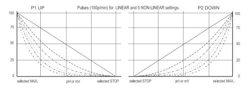
FIG 21 Non-linear pulsing of P1 and P2.
