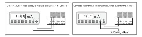
FIG 8 Calibrating 4-20mA with a multimeter.
