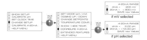
FIG 15 Configuration of 4-20mA range.
